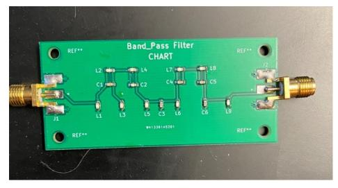
• Filter 2b (bpf\_2b): One of the filters from version 2 of what Nahum built
