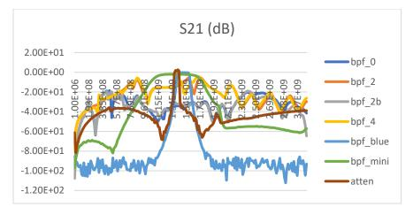
S21 is the signal going from Port 1 of the VNA, through the filter, and into Port 2.
