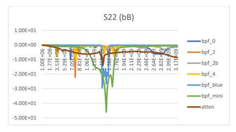
S22 is the signal going from Port 2 of the VNA, to the filter, and back to Port 2.
