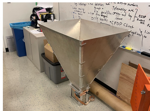
Figure 1: Left: Block diagram of CHART. Right: Sheet metal CHART horn antenna.
