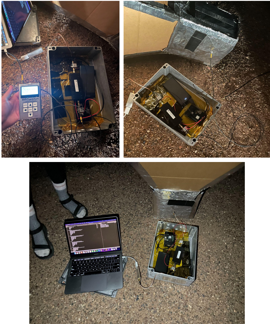
Figure 2. ( top left ) Our first calibration measurement was a sanity check with a signal generator. ( top right ) We considered using a longer RF cable to be able to move our box of electronics further from the antenna, but found that the longer cable introduced too much loss. ( bottom ) Our final measurement setup, with short cables to avoid signal loss as much as possible.
